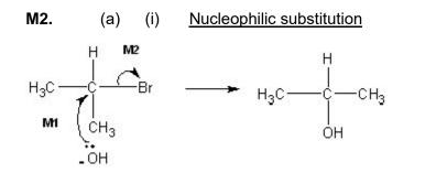
**M1** must show an arrow from the lone pair of electrons on the oxygen atom of the negatively charged hydroxide ion to the central C atom.
