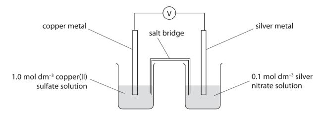
At 298 K, the emf of this cell was +0.40 V. The electrode potential of the copper metal / copper(II) ion electrode is +0.34 V. What is the electrode potential of this silver metal / silver(I) ion electrode?
