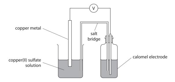
Under standard conditions, the emf of this cell was -0.07 V. The standard electrode potential of the copper metal / copper(II) ion electrode is +0.34 V. Hence the standard electrode potential of the calomel electrode is
