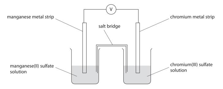
The standard electrode potential of the chromium(III)/chromium half cell is  $-0.74 \, \text{V}$  and that of the manganese(II)/manganese half cell is  $-1.19 \, \text{V}$ . Thus the emf of the cell, as shown in the diagram, under standard conditions is
