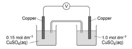
The student recorded an initial voltage of +0.16 V at 25 °C
