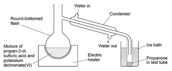
There are **three** problems with the apparatus set up in the figure above.
