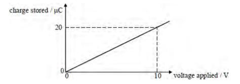
The energy stored, in  $\mu$ J, when the potential difference across the capacitor is 5 V, is
