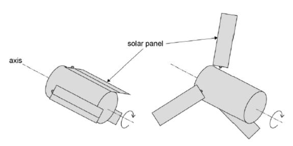
Just before it is released into space, the satellite is spun to rotate at 5.2 rad s<sup>-1</sup>. Once released, the solar panels are extended as shown in **Figure 2**.
