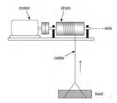
The drum, axle and other rotating parts have a moment of inertia about the axis of rotation of  $7.4 \text{ kg m}^2$ , and the mass of the load is 85 kg. The drum has a radius of 0.088 m.
