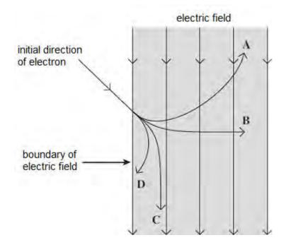
**Q21.**The diagram shows a negative ion at a point in an electric field, which is represented by the arrowed field lines.
