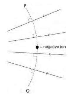
**Q5.**The diagram shows a small negative charge at a point in an electric field, which is represented by the arrowed field lines.
