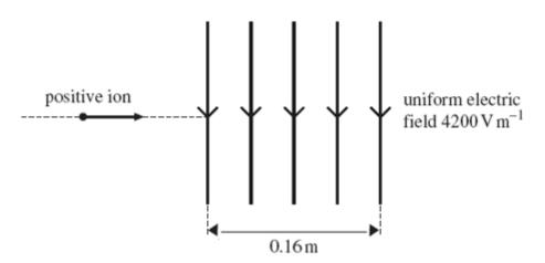
An ion carrying a charge of  $+4.8 \times 10^{-19}$ C travels horizontally at a speed of  $8.0 \times 10^{5}$ ms<sup>-1</sup>. It enters a uniform vertical electric field of strength 4200 V m<sup>-1</sup>, which is directed downwards and acts over a horizontal distance of 0.16m. Which one of the following statements is **not** correct?
