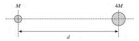
The resultant gravitational field strength is zero along the line between their centres at a distance y from the centre of the star of mass M.
