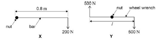
What is the minimum length l of the wrench which would be needed for him to loosen the nut?
