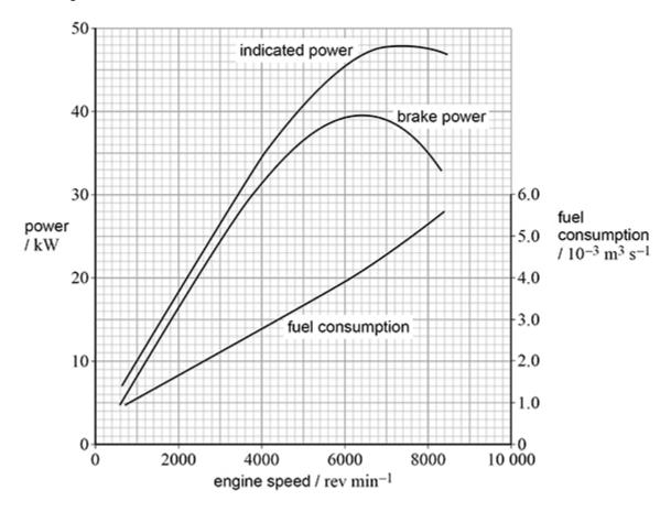
The figure above shows how the indicated power, brake (or output) power and fuel consumption of the engine vary with the engine speed. The scale on the left-hand axis is power and the scale on the right-hand axis is fuel consumption.
