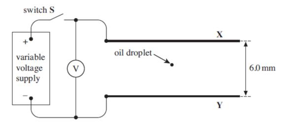
(a) (i) With the switch **S** open, the droplet fell vertically at a constant velocity of  $1.1 \times 10^{-4}$  ms<sup>-1</sup>. Show that the radius of the droplet is about  $1.0 \times 10^{-6}$  m. Assume the droplet is spherical.
