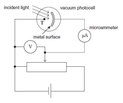
(a) The potential of the metal surface may be changed by adjusting the potential divider. Explain why the microammeter reading decreases when the metal surface is made more positive relative to T.
