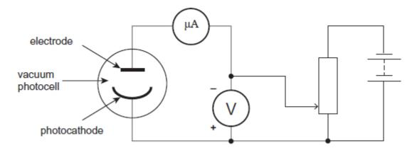
Monochromatic light falls on the photocathode. A current is recorded when the potential difference (pd) between the photocathode and the electrode is zero.
