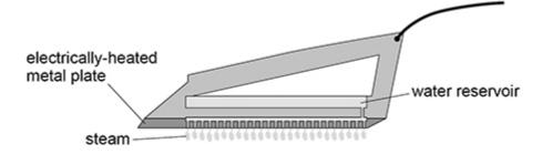
Water from a reservoir drips onto an electrically-heated metal plate. The water boils and steam escapes through holes in the metal plate.
