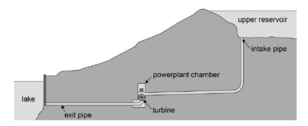
Water from the upper reservoir is to fall through a vertical distance of 90 m before reaching a powerplant chamber. The water rotates a turbine in the chamber that drives an electricity generator. After leaving the turbine, the water travels through an exit pipe to a lake.
