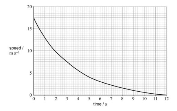
(a) Determine the force decelerating the vehicle 2.0 s after entering the escape lane.
