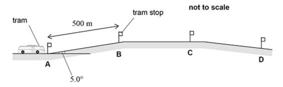
The tram must travel 500 m along this incline on one charge of energy.
