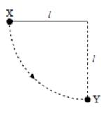
A ball of mass m, which is fixed to the end of a light string of length l, is released from rest at X. It swings in a circular path, passing through the lowest point Y at speed v. If the tension in the string at Y is T, which one of the following equations represents a correct application of Newton<sup>II</sup>s laws of motion to the ball at Y?
