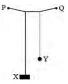
**X** is a heavy pendulum, the frequency  $f_x$  of which can be varied. **Y** is a lighter pendulum of fixed frequency  $f_y$ . As the frequency of oscillation of **X** is increased by shortening the thread, the amplitude of the oscillation of **Y** changes.
