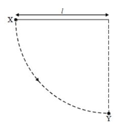
A simple pendulum consists of a bob of mass m on the end of a light string of length I. The bob is released from rest at X when the string is horizontal. When the bob passes through Y its velocity is v and the tension in the string is T. Which one of the following equations gives the correct value of T?
