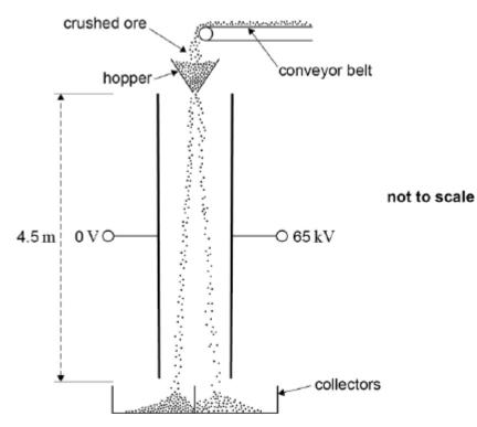
The crushed particles of the two different minerals gain opposite charges due to friction as they travel along the conveyor belt and through the hopper. When they leave the hopper they fall 4.5 metres between two parallel plates that are separated by 0.35 m.
