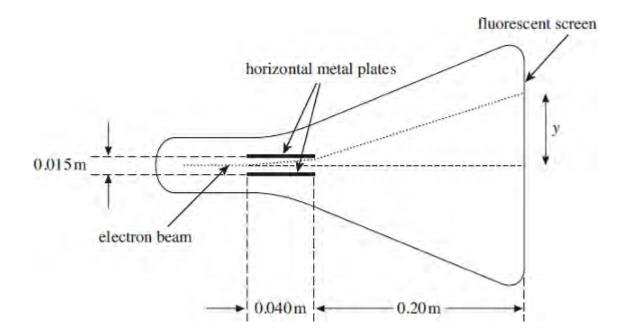
The electron beam passes between two horizontal metal plates and goes on to strike a fluorescent screen at the end of the tube. The plates are 0.040 m long and are separated by a gap of 0.015 m. A potential difference of 270 V is maintained between the plates. An individual electron takes  $1.5 \times 10^{-9}$  s to pass between the plates. The distance between the right-hand edge of the plates and the fluorescent screen is 0.20 m.
