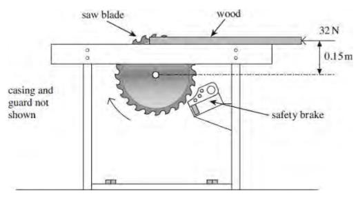
A horizontal force of 32 N is needed to push a piece of wood into the saw. The force acts on the blade at an effective radius of 0.15 m.
