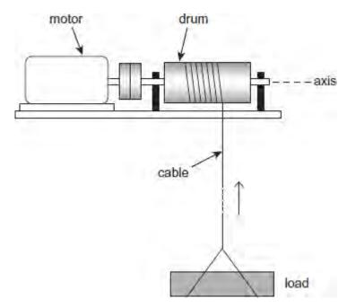
The drum, axle and other rotating parts have a moment of inertia about the axis of rotation of 7.4 kg  $m^2$ , and the mass of the load is 85 kg. The drum has a radius of 0.088 m.
