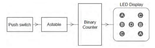
The binary counter consists of three rising edge triggered D-type flip-flops. The counter outputs are X, Y and Z. The most significant bit is Z.
