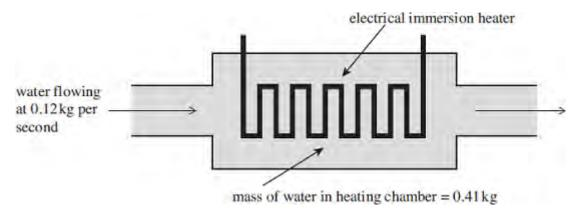
(a) Assuming all the energy is transferred to the water, calculate the rise in temperature of the water as it flows through the heater.
