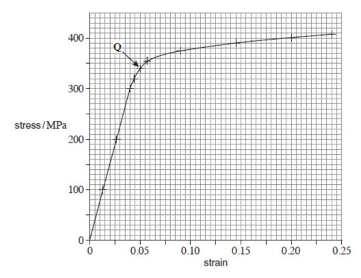
(i) The engineer has labelled a point  $\mathbf{Q}$  on the graph. This is a point beyond which the behaviour of the material changes irreversibly. State the name for this point.
