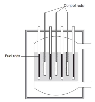
The control rods, made from boron, are used to control the chain reaction. Boron atoms absorb neutrons without undergoing nuclear fission.
