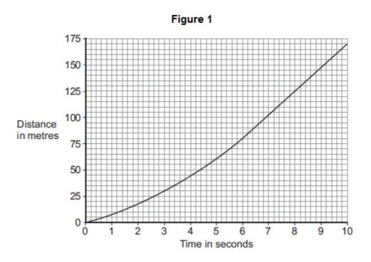
Use **Figure 1** to calculate the maximum speed the car was travelling at. Show clearly how you work out your answer.
