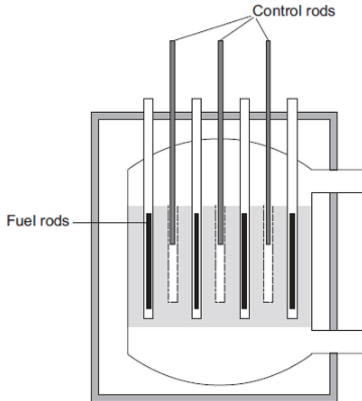
The control rods, made from boron, are used to control the chain reaction. Boron atoms absorb neutrons without undergoing nuclear fission.
