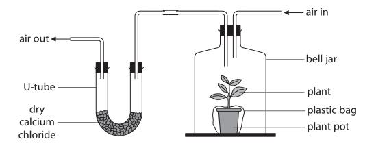
The calcium chloride absorbs the water lost by the plant.
