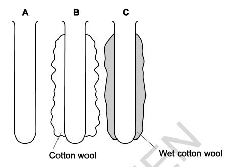
Test tube A has no insulation. Test tube B is wrapped in cotton wool. Test tube C is wrapped in wet cotton wool.
