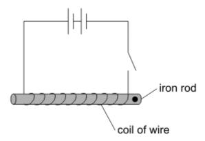
When the switch is closed the iron rod becomes an electromagnet. Give **two** ways Hannah could make the electromagnet stronger.
