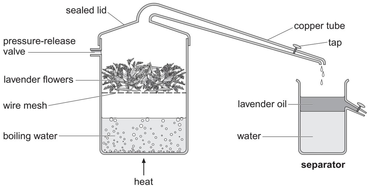
Water vapour and lavender oil vapour pass down a copper tube towards a separator.
